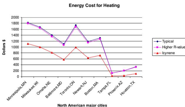
Figure 2.1 shows the energy costs for heating in several different cities throughout North America. The heating costs are compared for the three different insulation systems. It can be seen that savings on heating cost reached up to 30%-40% with Icynene® when compared to the “Base Case” and “Higher R-Value” insulation systems. Also, the graph indicates that the colder the climate, the greater the heating cost savings are with Icynene®.
